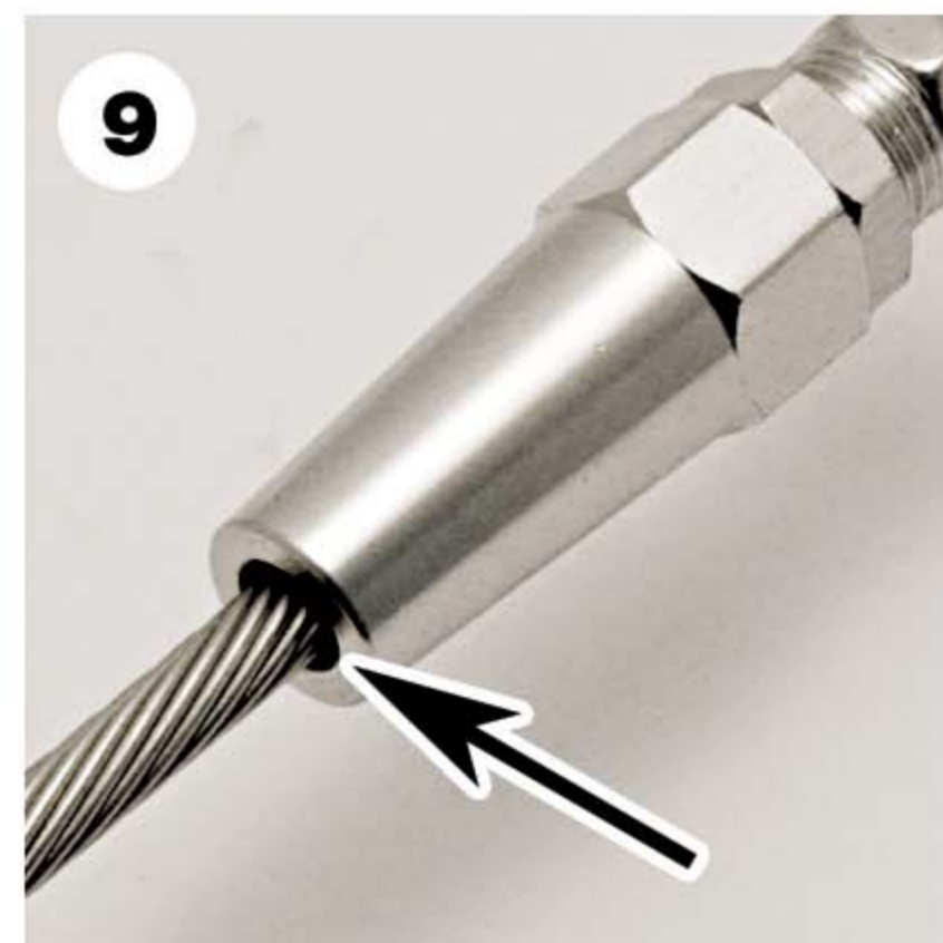
9. Suncor recommends sealing with a Non-Acidic silicone (Seka Flex) sealing compound. Place sealant in the tip of the Cone around the wire.
